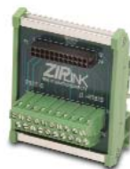
ZL-RTB20 20-pin feed-through connector module
