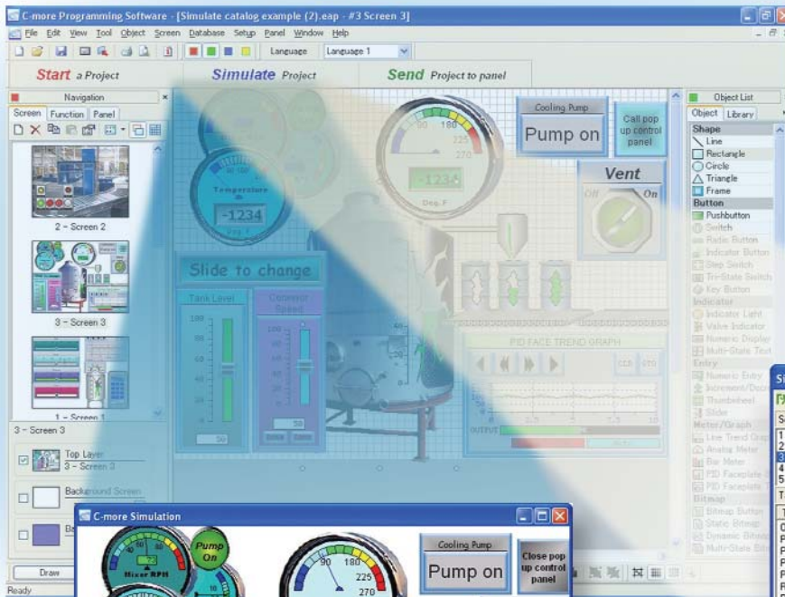
The simulation control window shows the list of screens and the tags and add their values on the highlighted screen in the list.
