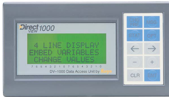
4-line by 16-character backlit LCD display
