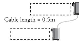
**\*Note:** The (-1) versions of the expansion cables pass 24 VDC through on an isolated wire. (All cables pass the 5 VDC base power.) Any local expansion DC input module configured for "internal power" (current sourcing) must either have a power supply preceding it on the same base or, have a (-1) version cable pass 24 VDC from a power supply on the preceding base.
